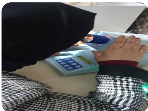
Fig (21): Determine the melting point.
